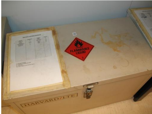
Storage container marked to show contents and hazard
