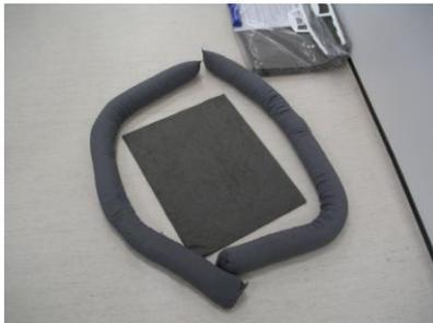
4. Deactivate the hazardous material by absorbing or neutralising appropriately. Leave absorbent material in place for at least 20 minutes.
