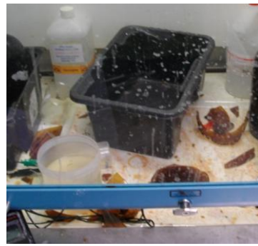
Winchester jar exploding due to severe over pressure caused by rapid gas generation
