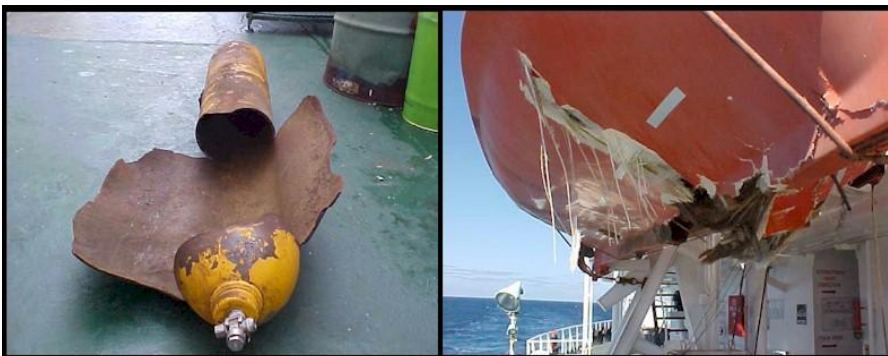
Effects of exploding gas cylinder on the hull of a lifeboat
