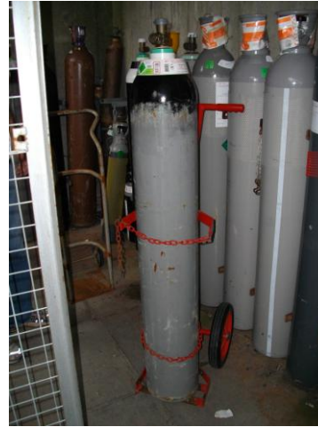
Both safety chains in place, regulator removed
