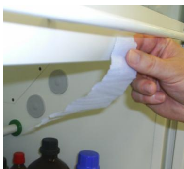
The direction of paper movement shows the air is being drawn into the Fume Hood
