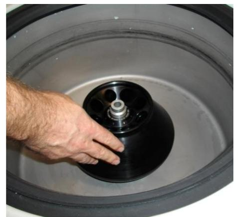
Gently spin the rotor to ensure the pins have located and the rotor moves freely
