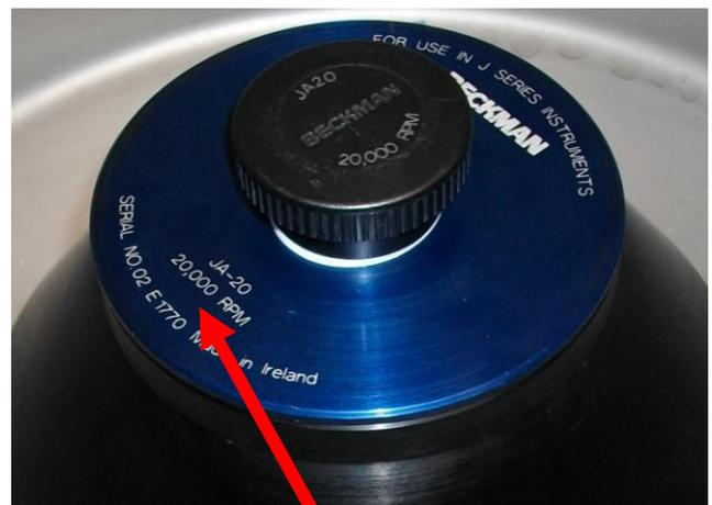
This shows maximum rotor speed of 20,000 RPM
