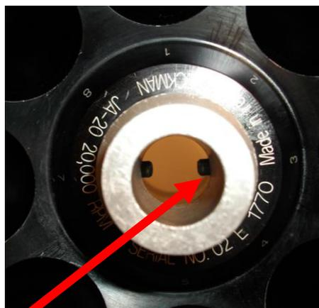
Ensure rotor pins are properly lined up with spindle pins
