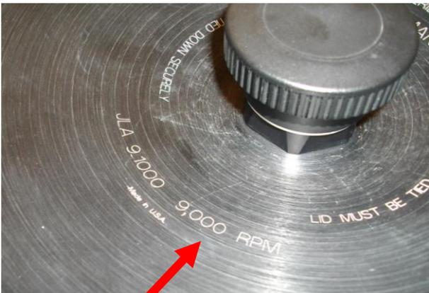
This shows maximum rotor speed of 9000 RPM
