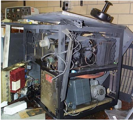
Centrifuge destroyed as a result of the wrong rotor being used
