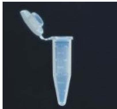
Tube that can be used in Centrifuge
