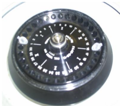
Rotor must be balanced
